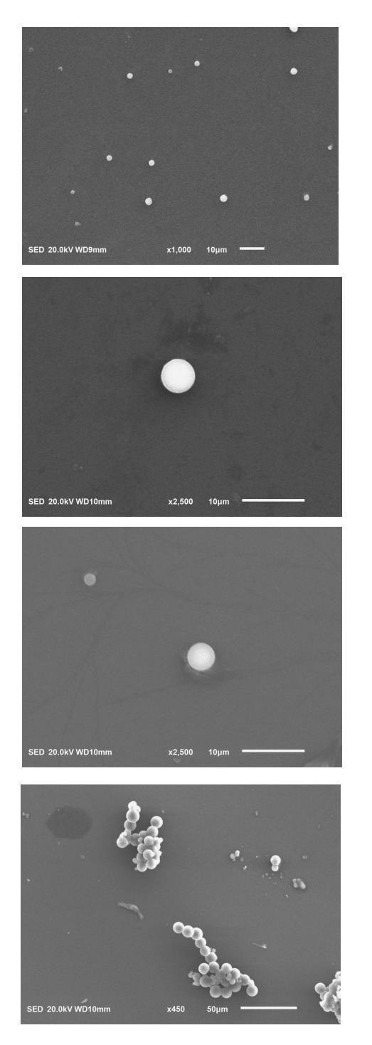
Outlet 1 Less and dispersed spheres Diameters ~2-3µm
